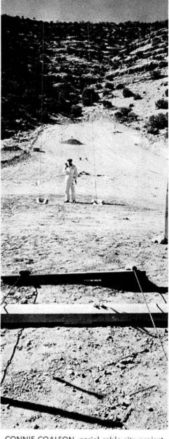
CONNIE COALSON, aerial cable site project engineer, stands at the impact point between the two cables which are attached to the test unit suspended 600 feet above from an overhead cable. The tow cables, which curve underground, can be seen coming out of the guide tubes, heading toward the rocket sled for attachment.
